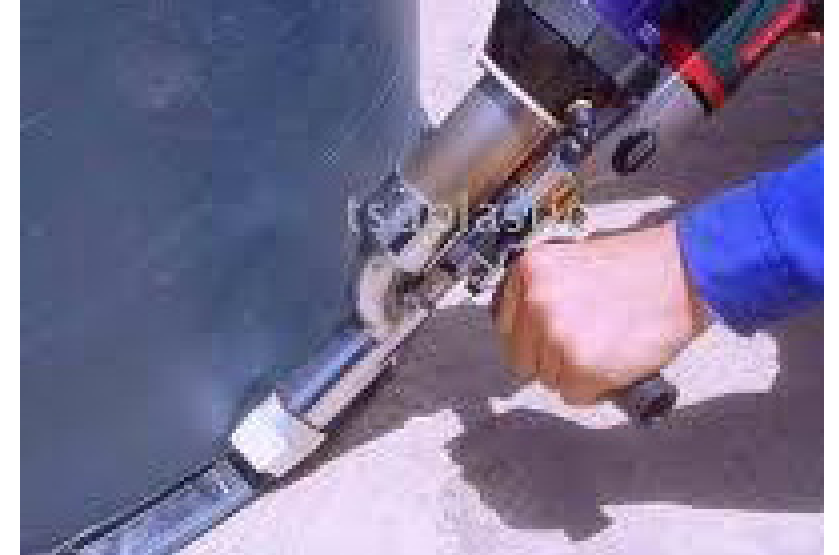
CONTINUOUS FEED PLASTIC ROD For heavier liners and custom factory fabricated boots.
